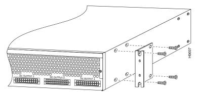
Note: The second bracket attaches to the other side of the chassis.
